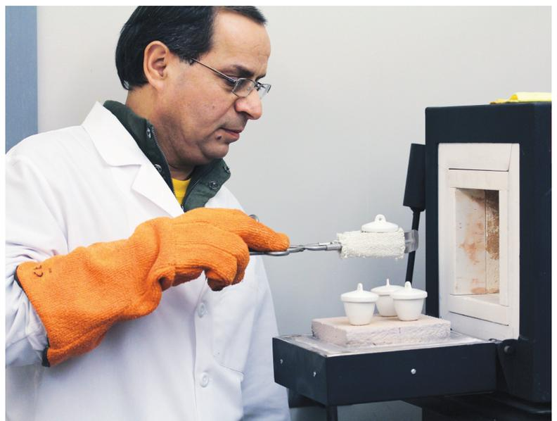
*Measuring the ash content, an indicator of the amount of inorganic filler in a glove: Dr. Amer Tiba removes porcelain crucibles from an ADA Laboratory oven heated at  $750 \pm 25^\circ\text{C}$  during gravimetric determination of total residual powder according to ASTM D6124-06.*
