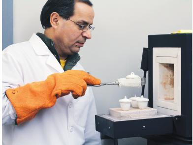
Measuring the ash content, an indicator of the amount of inorganic filler in a glove: Dr. Amer Tiba removes porcelain crucibles from an ADA Laboratory oven heated at 750±25°C during gravimetric determination of total residual powder according to ASTM D6124-06.
