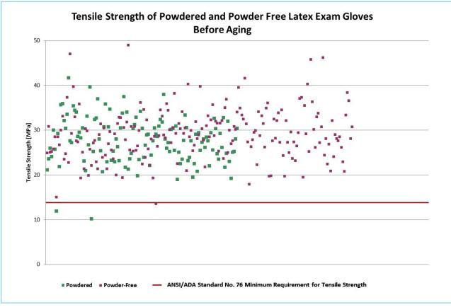
Figure 1. Plot of tensile strength values for powdered and powder-free gloves before aging
