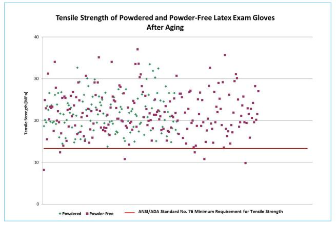
Figure 2. Tensile strength of powdered and powder-free latex exam gloves after aging.
