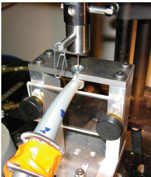
Figure 9B. Sample picture of extraction force fixture mounted to the mechanical testing system frame with handpiece positioned for a dynamic extraction force test.
