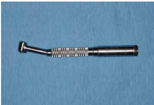
Figure 2. Borden Airotor high-speed air-turbine handpiece. Photograph reproduced with permission of Dentsply International, York, Pa.
